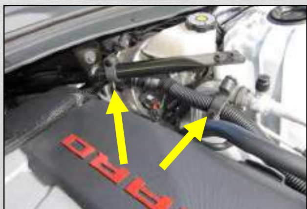
7. Locate the upper half of the resonator tube near the master cylinder and disconnect the tube retainers on the strut tower brace and the A/C line.
