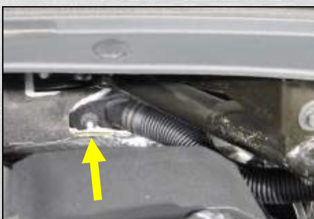
8. At the firewall, remove the 6mm flange nut at the resonator tube base. Turn the tube 1/4 turn Clockwise and remove it from the vehicle.
