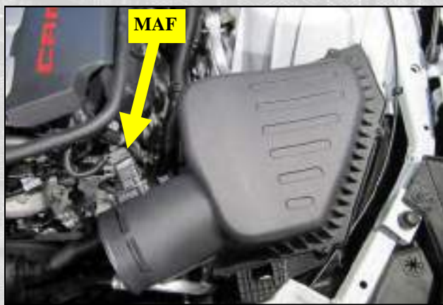
4. Disconnect the air flow meter, or MAF, in the air box lid and remove the entire airbox assembly from the vehicle.
