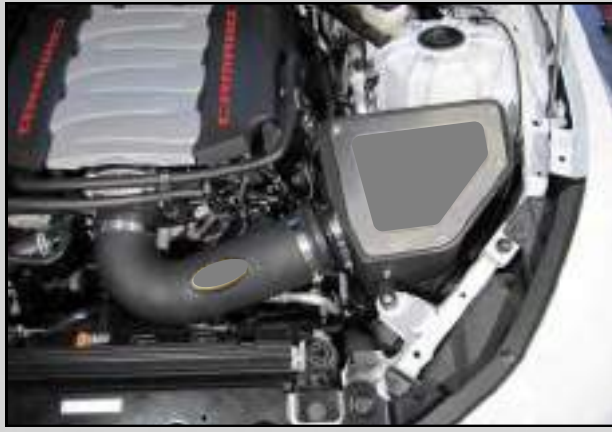
26. Slowly lower the hood to test clearances. Make sure all clamps, hoses, bolts, and screws are tight. Double check the hood clearance. Reconnect the negative battery terminal and re install the access panel.
