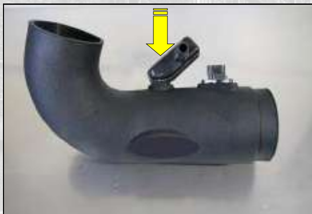
16. Transfer the PCV fitting into the Grommet in the StreetFighter Performance Airbox Intake Tube.
