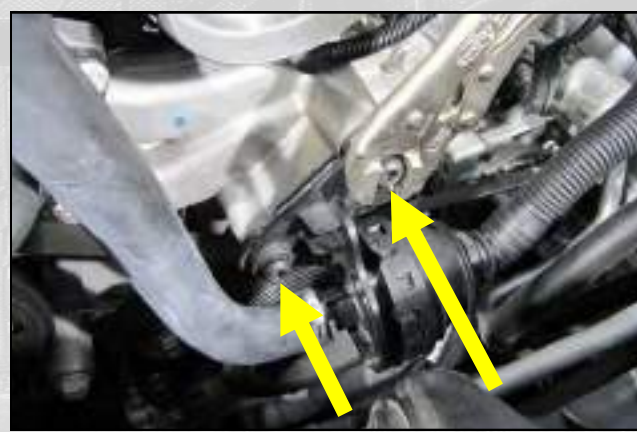
6. Remove the two bolts in the resonator diaphragm bracket using a T-50 Torx bit or with a pair of locking pliers as shown. The resonator, bolts and bracket will not be used with the StreetFighter Performance Airbox.
