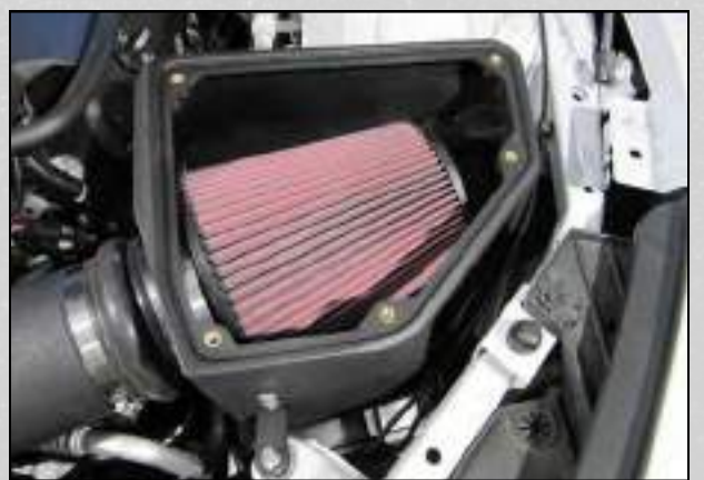
23. Install the StreetFighter Premium Airfilter on to the Fitted Adapter in the Airbox.
