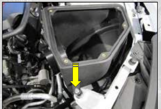
17. Place the Airbox assembly into the engine compartment as shown, with the mounting posts only fully seated in all three grommets.
