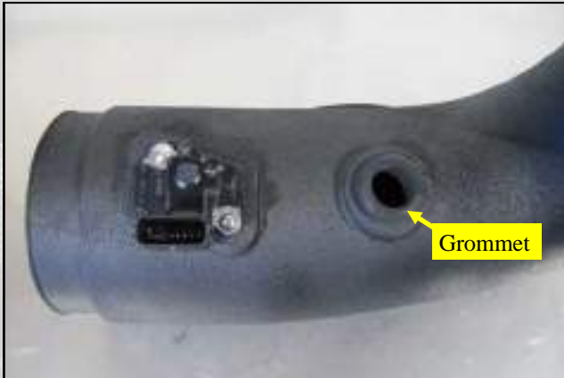
14. Transfer the MAF Sensor from the factory airbox, into the Intake Tube and secure it using the supplied #8 Button Head Screws. Insert the Grommet into the Intake Tube as shown.
