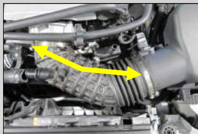
3. Loosen the clamps on both ends of the intake tube and remove it from the vehicle.
