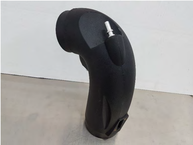
13. Insert the remaining Grommet and Fitting into the Intake tube as shown.
