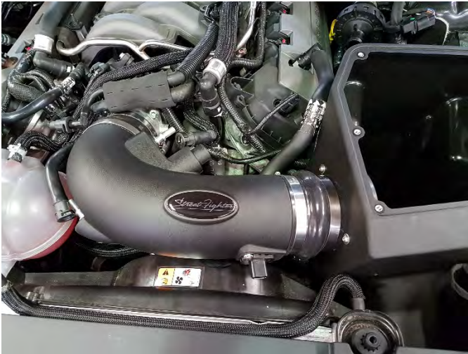
15. Insert the Intake Tube into the Hump Hose and Reducer then tighten all 4 Intake Clamps.
