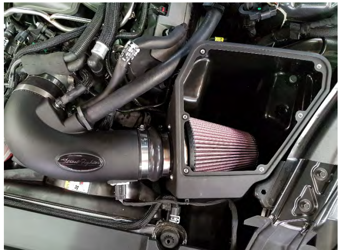
18. Install the Premium Filter onto the Filter Adapter inside of the Airbox.
