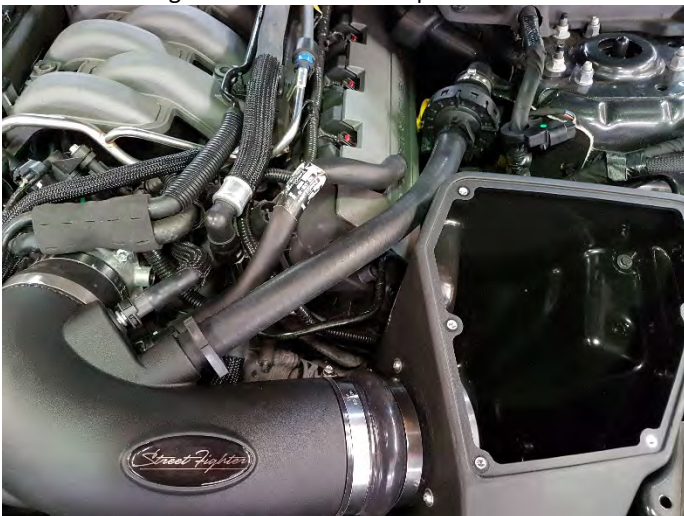
17. Connect the resonator to the Intake Tube as shown using the supplied 1" Hose and the Speed clamps on both ends.
