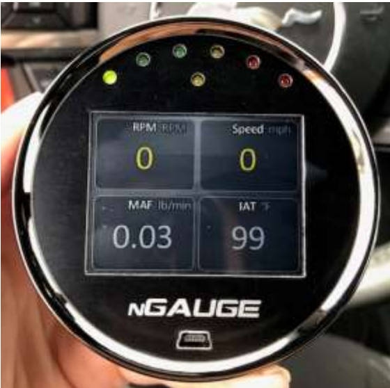
Select which signal of the four you would like to replace with Oil Pressure for this example we will replace the IAT.
