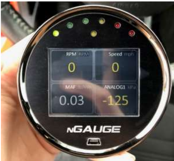
You should now see the ANALOG1 on the screen, select the "ANALOG1" signal
