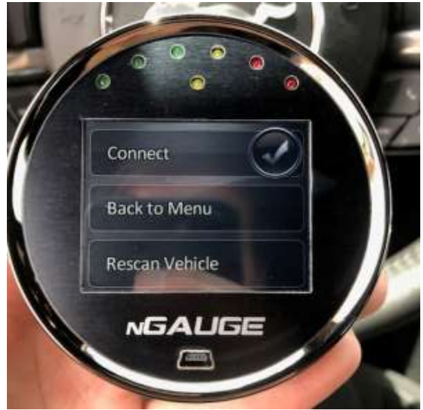
Select "Connect" at this point you need to turn the car ignition on.
