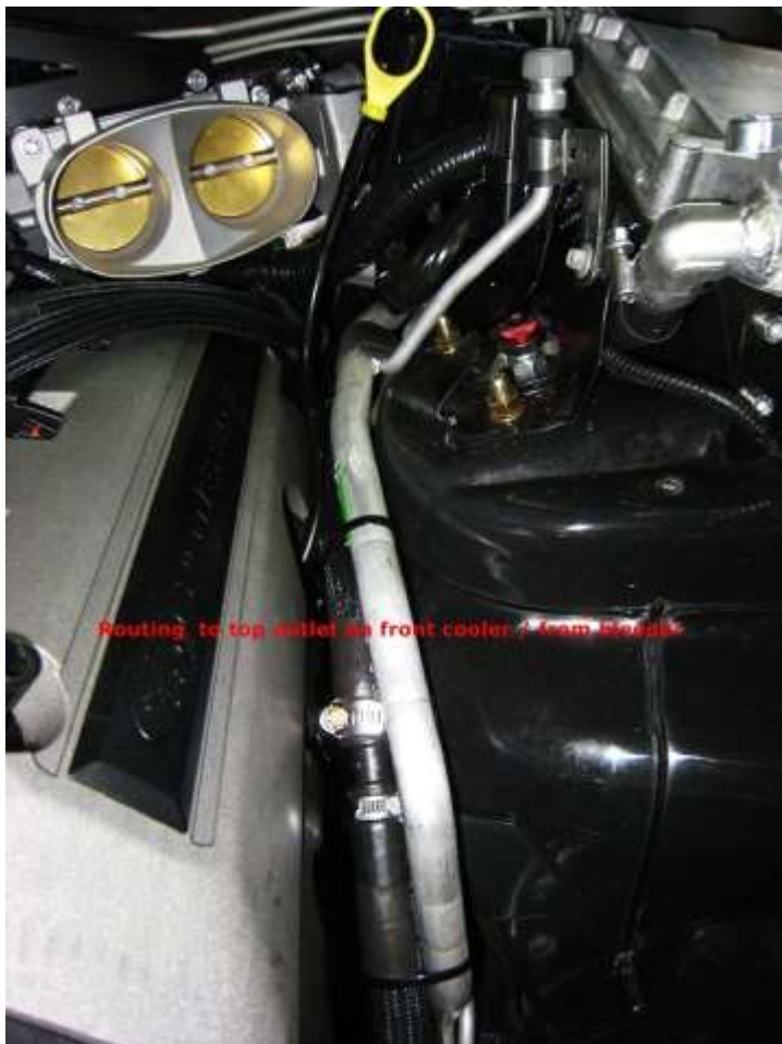
L/H Hose Routing along A/C pipe
